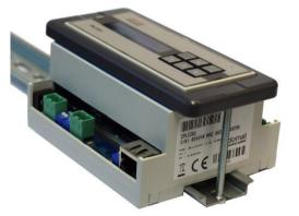
Summary The mounting FRAME for fixing of the MiniPLC into front panel. Cut a 106 x 46 mm aperture and two holes for the screws in the front door, then use a 150 mm DIN rail to mount the MiniPLC from inside. The frame covers the aperture on the outer side.
